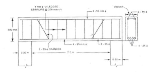
**2)** Prepare the Bar bending schedule of a simply supported R.C.C. Lintels from the following specification:
