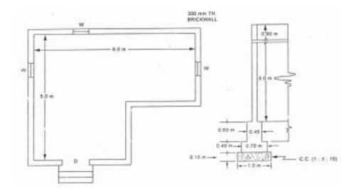
Calculate the following quantities by a) central line method b) Long wall & shortwall method.
